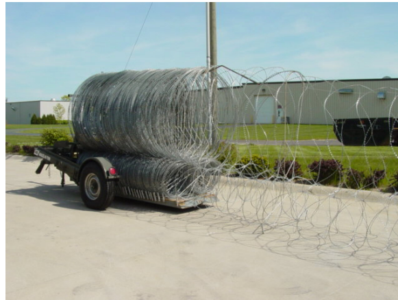
Figure 2: Wire Barrier System being deployed
