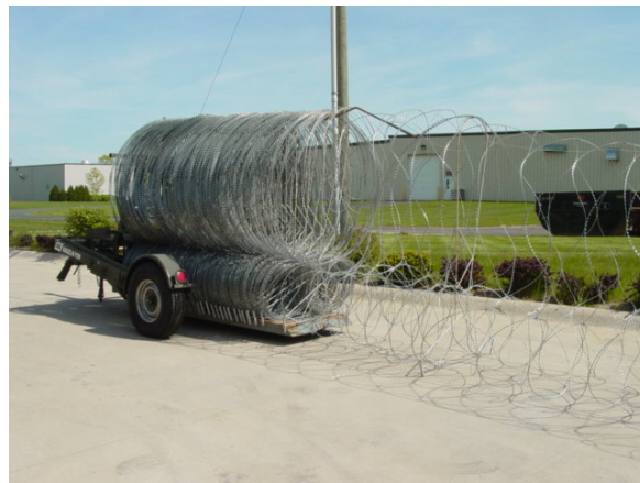
Figure 2: Wire Barrier System being deployed
