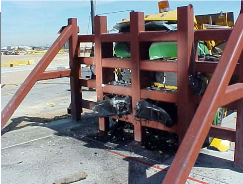
After the crash test, this Gate was still completely operational.
